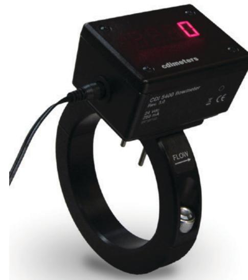
The CDI 5400 clamps onto a pipe, with two flow-sensing probes projecting into the pipe through 3/16-in. drilled holes. It seals directly to the pipe; no cutting or welding is required for installation. Because each flowmeter is made and calibrated for a specific size of pipe, the digital display indicates flow directly, with no setup or adjustment.
