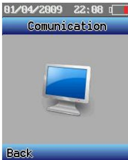
This function is that take the instrument memory as a virtual USB disk, computer can upload or download components data and measuring curve data, do not have to install driver.
