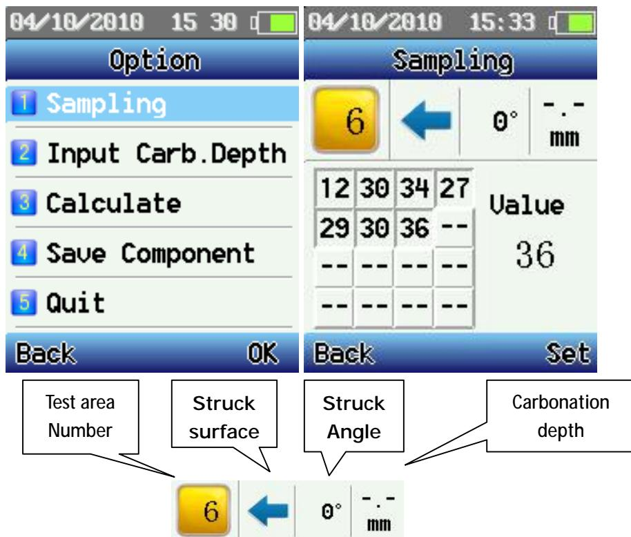
Enter **【Sampling】** interface to begin measuring, if need set impact surface and impact angle and carbonation depth of the test area, choose **Set** and the parameter interface will appear. We can set test area parameter, change parameter or delete test values in it.
