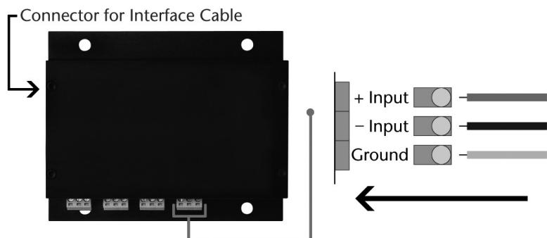
*Warning: Note the polarity instructions. Do not attach wires to the wrong terminals.*
