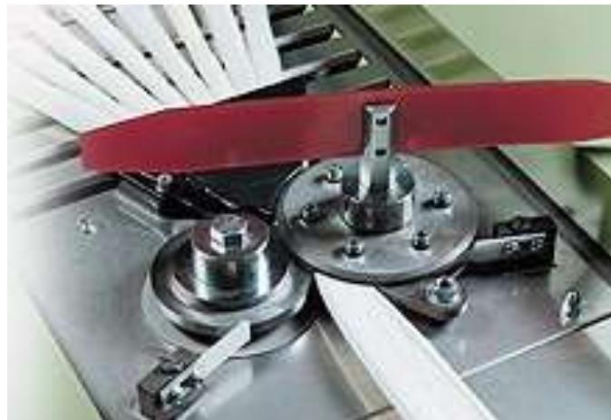
*The constant thickness of the yarn during the yarn production for textiles is decisive for the quality. Eddy current sensors at the web infeed which measure the thickness using sensing rollers are used for this. Another eddy current sensor monitors the already corrected thickness.*
