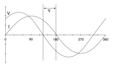
The power factor is the cosine of the phase angle  $\phi$  between current and voltage, improving it enables you to use energy more efficiently and cut power costs.
