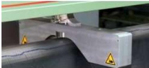
*The profilometer of the thicknessCONTROL.TTP series accurately measures the thickness profile of tire tread or side walls during the extrusion process and enable therefore an efficient control during production as well as a fully recorded quality control.*
