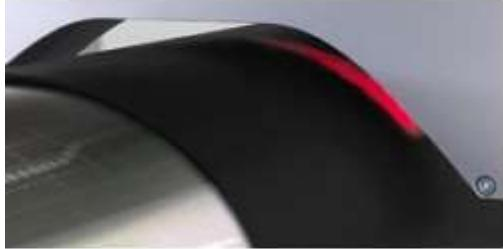
*For tire production, tread strips are cut from the extruded strip material. The system TLS 8303.I is applied in the extrusion line to measure the length of the strips immediately after the cutting machine in order to ensure a secure production process in high quality.*
