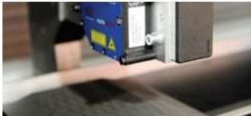
*The profilometer thicknessCONTROL TTP 8302.T is applied for sampling regarding the extrusion process of treads, side wall and inner liner material. The system offers measuring results in high precision and allows therefore an efficient production as well as a fully recorded quality control.*
