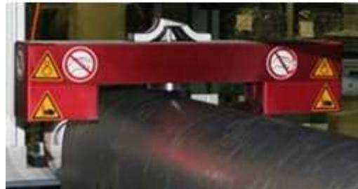
*During the production of inner liner, the thickness profile of inner liner material is measured immediately after the calender using systems of the thicknessCONTROL TIP series. Accurate precision of the non-contact optical system ensures high quality and security of the product produced. Sensors belonging to the thicknessCONTROL RTP series can also be applied for this application.*
