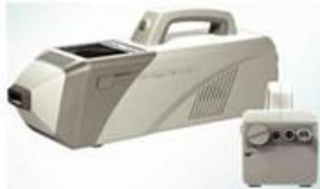
*The application of pseudo random sequence ion open technology and Hardmard algorithm technology improves the signal-to-noise ratio and anti-interference ability of the detector and reduce the rate of false alarms. The design of the sampling pen prevent the pollution of the test paper. Black powder, ammonium nitrate amine, TNT, AN-TNT, RDX, peptamine , HMX, CE, C4, etc., and may add a new sample according to need at any time.*
