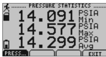
Displays statistics (maximum recorded value, minimum recorded value, and average recorded value) for the pressure channel.
