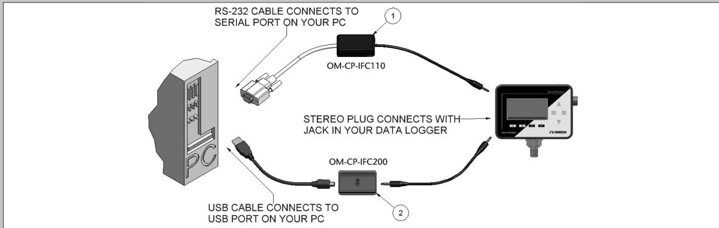
1. Fully insert the male connector of the OM-CP-IFC110 interface cable into the female receptacle of the data logger. Insert fully the RS232 connector into the Serial Port.
