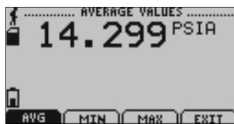
Displays statistics from the pressure channel sorted by type (maximum recorded value, minimum recorded value, or average value).
