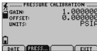
*Displays calibration information for pressure channel.*
