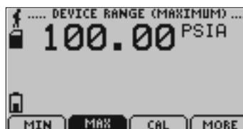
Displays values indicating maximum pressure detectable by the OM-CP-PR2000.
