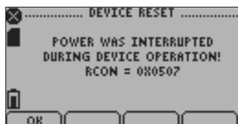
Displayed as notification when power is interrupted during device operation.
