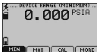
Displays values indicating minimum pressure detectable by the OM-CP-PR2000.
