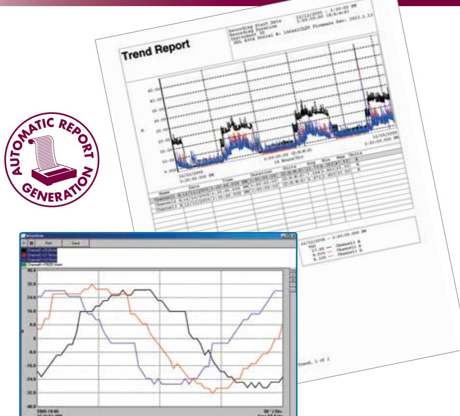
Real-time display of all active inputs on computer through DataView® software.
