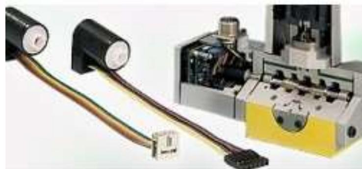
*Servo and proportional valves regulate the volume flow in hydraulic systems. Displacement sensors are necessary for precise control. Inductive displacement sensors mounted on a pressure tube outside the pressure section are used for this. From this position, they measure on the piston through the pressure tube for an exact regulation.*
