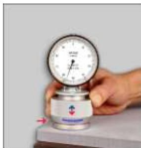
**Durometer according ISO 7619-1 for determining the Shore surface hardness of foams, steering wheels and inner linings of motor vehicles with hardness < 20 Shore A**
